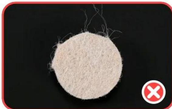
The felt pad after peeling off is irregular and the felt is loose
