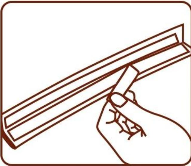
Attach the adhesive tape to the inside of the edge guard
